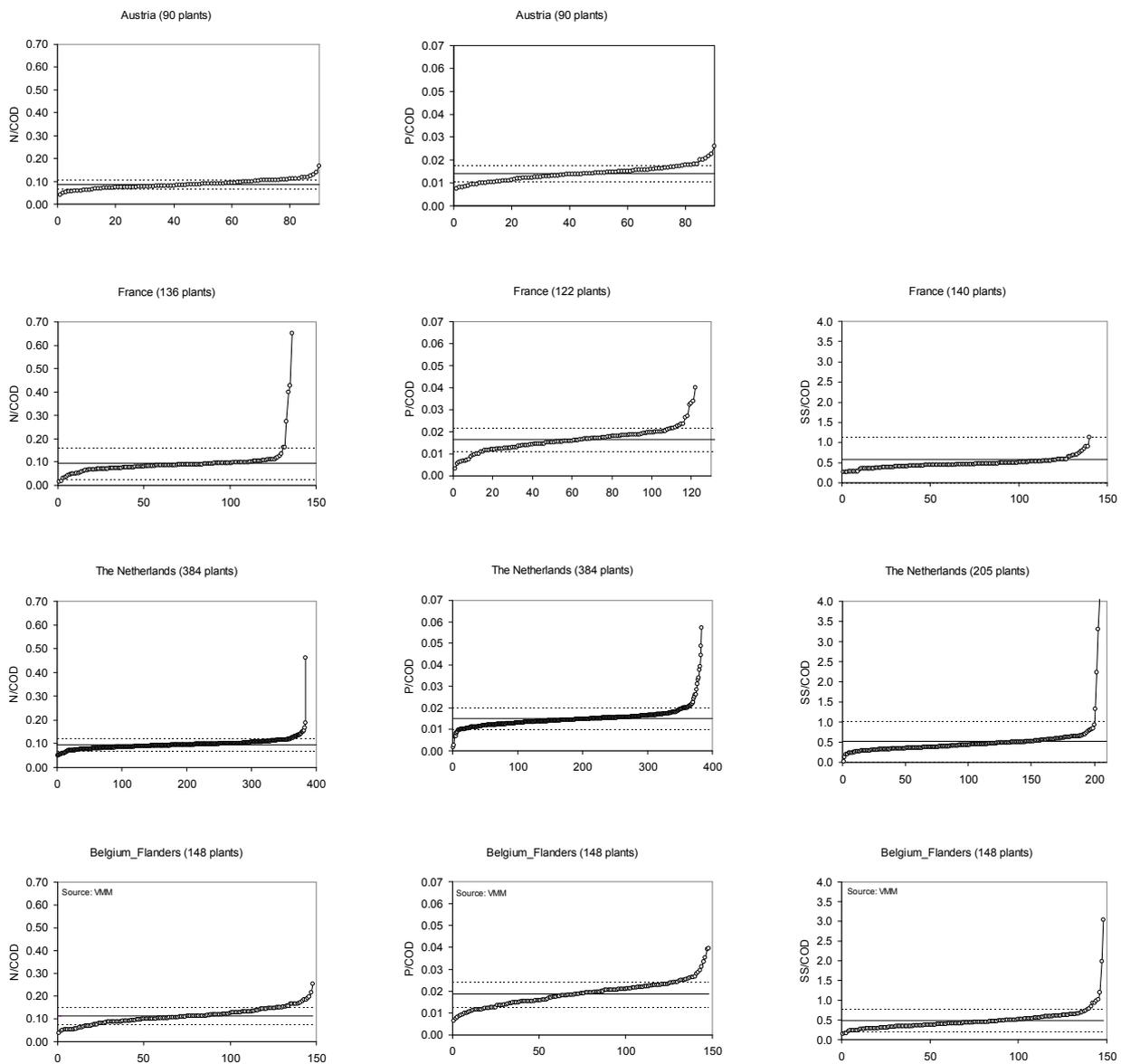
**Figure 1:** Comparison of the distribution of N/COD, P/COD and SS/COD for municipal wastewater (—) average value, (- - -) average value  $\pm$  standard deviation. The number of wastewater treatment plants having provided data is indicated for each case.
